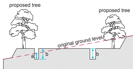
Figure 3: Levels from which foundation depths are measured where trees or hedgerows are proposed
